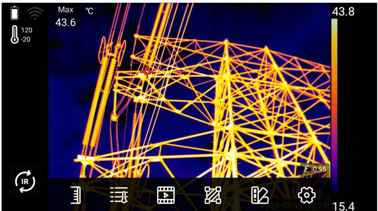
Click system menu button
