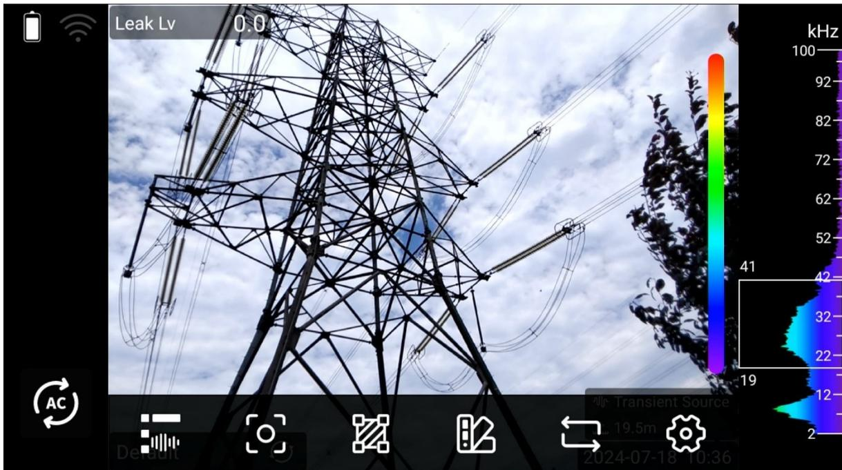
Includes: acoustic parameters, focus mode, measurement tool, palettes, detection mode, settings
