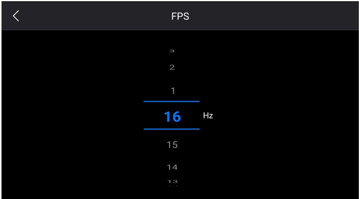
1. The recording frame rate can be set between 1~16 frames, and the shooting mode is automatically selected as video recording after selection;
