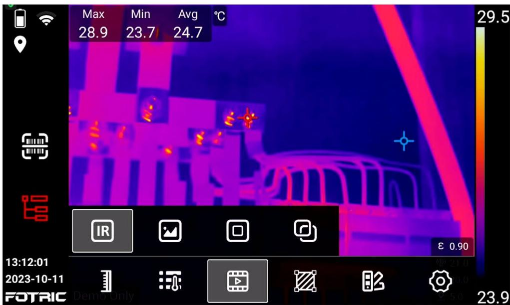
! Note: In thermal image mode, please make sure that the infrared acoutherm imager is accurately focused. If the infrared thermal image is not clearly focused, it will affect the accuracy of the acoutherm imager's temperature measurement.
