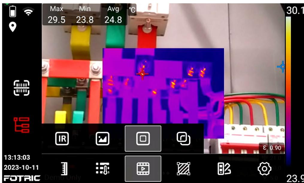
2-When focusing the acoutherm imager automatically adjusts the position of the thermal image to automatically match the visible light.
